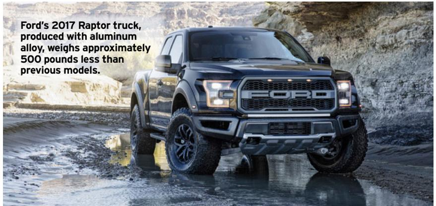
**Ford's 2017 Raptor truck, produced with aluminum alloy, weighs approximately 500 pounds less than previous models.**
